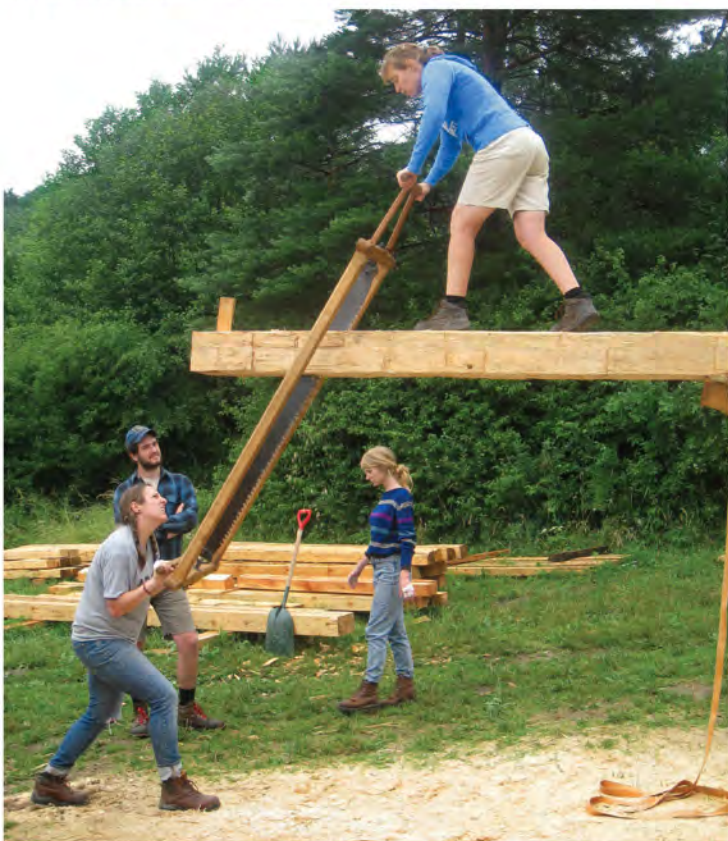
8–11 Clockwise from top left, deep-scoring oversize logs, joggling large chips, hewing to the line quad-teaming fashion and, at left, turning to another trade, trestle-sawing to get out smaller stuff from hewn baulks.
